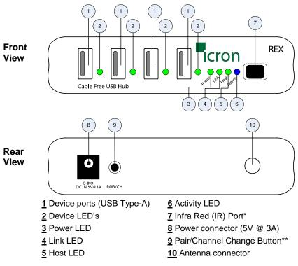
\* IR port used to pair the LEX unit and the REX unit only
